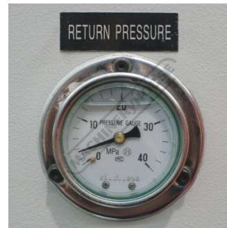
Return Pressure Gauge
