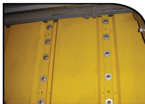
Full length back sheet supports with roller balls
