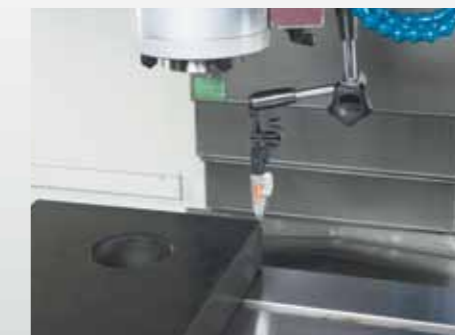
Right angle test on X and Y axes
