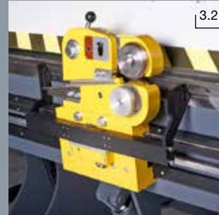
3.1 SL shears / 3.2 SLE shears / 3.3 SL3 shears All bending machines can be equipped with a SL/SLE shearing system for 1.5 mm steel sheets or a SL3 for 3 mm sheets. With the SLE and SL3, the air gap and the overlap can be set for various steel sheet thicknesses.
