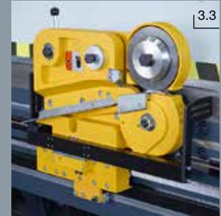
3.1 SL shears / 3.2 SLE shears / 3.3 SL3 shears All bending machines can be equipped with a SL/SLE shearing system for 1.5 mm steel sheets or a SL3 for 3 mm sheets. With the SLE and SL3, the air gap and the overlap can be set for various steel sheet thicknesses.
