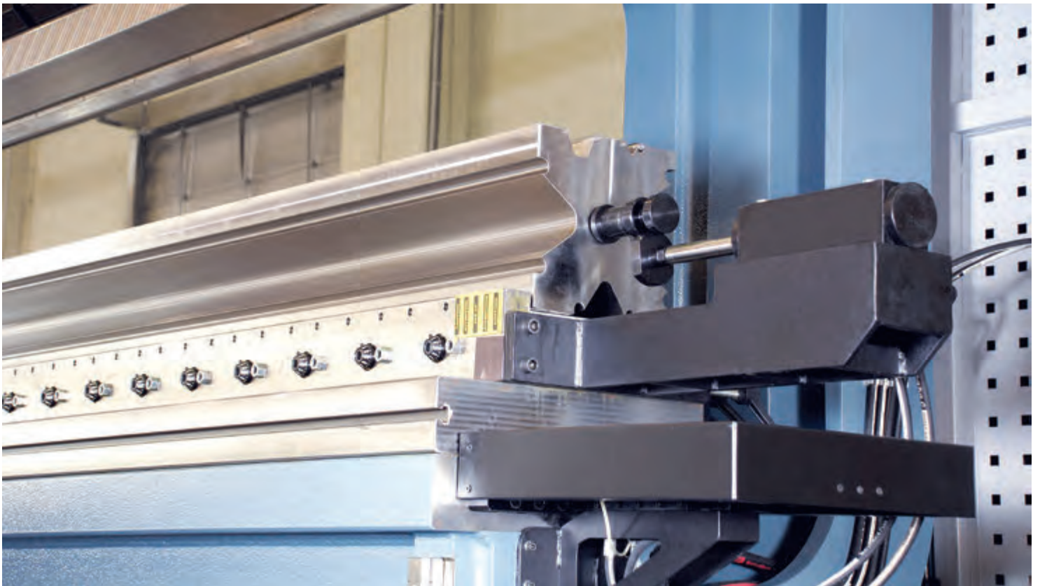
Hydraulics Bottom Tool Separation System
