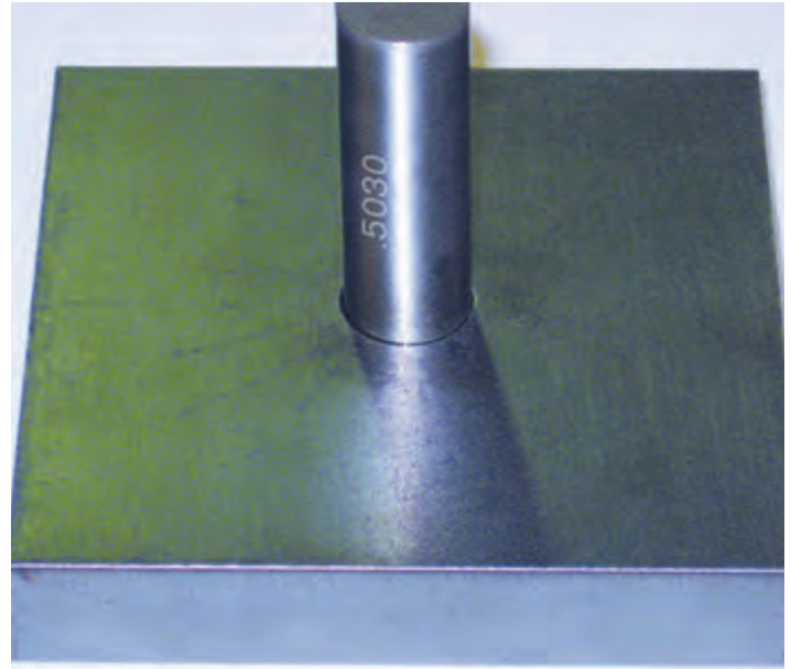
1 2 hole with True Hole technology cut with HPRXD Plasma
