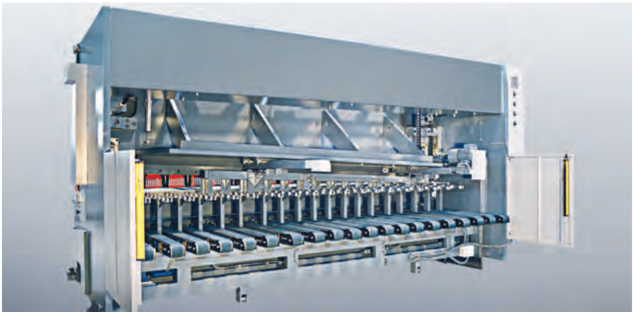
Sheet Support Devices with Conveyor and Scrap Container
