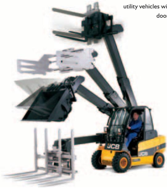
Changing attachments on ordinary masted lift trucks is usually time consuming and difficult. Usually it's not worth all the trouble. But on a JCB Teletruk you can change from forks to shovel in less than 20 seconds without leaving the cab.
