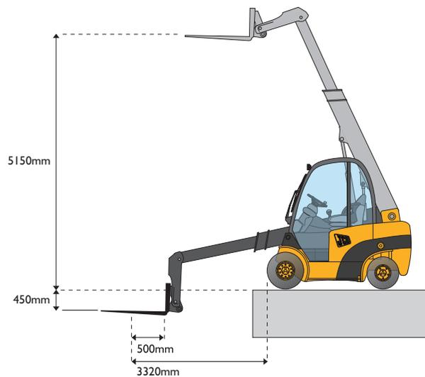
Ordinary lift trucks use hydraulic power for the lift cycle only, and then gravity to lower. But the JCB Teletruk uses full hydraulic power down too; and this can be put to good use for specialist applications such as loading ships stores.
