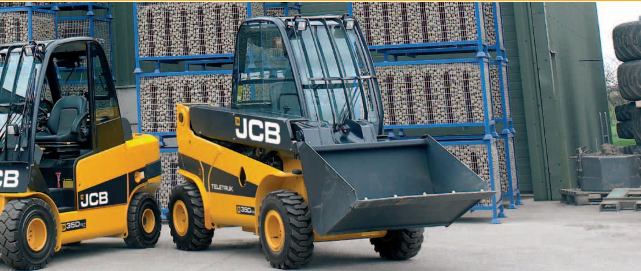
most versatile small counterbalanced lift truck. The JCB Teletruk is not just another lift truck. The range covers the most popular 2.5t – 3.5t capacity bands; diesel-powered two-wheel drive or four-wheel-drive, and two-wheel drive gas models. Teletruk is a true industrial counterbalanced machine. Because there's no vertical
