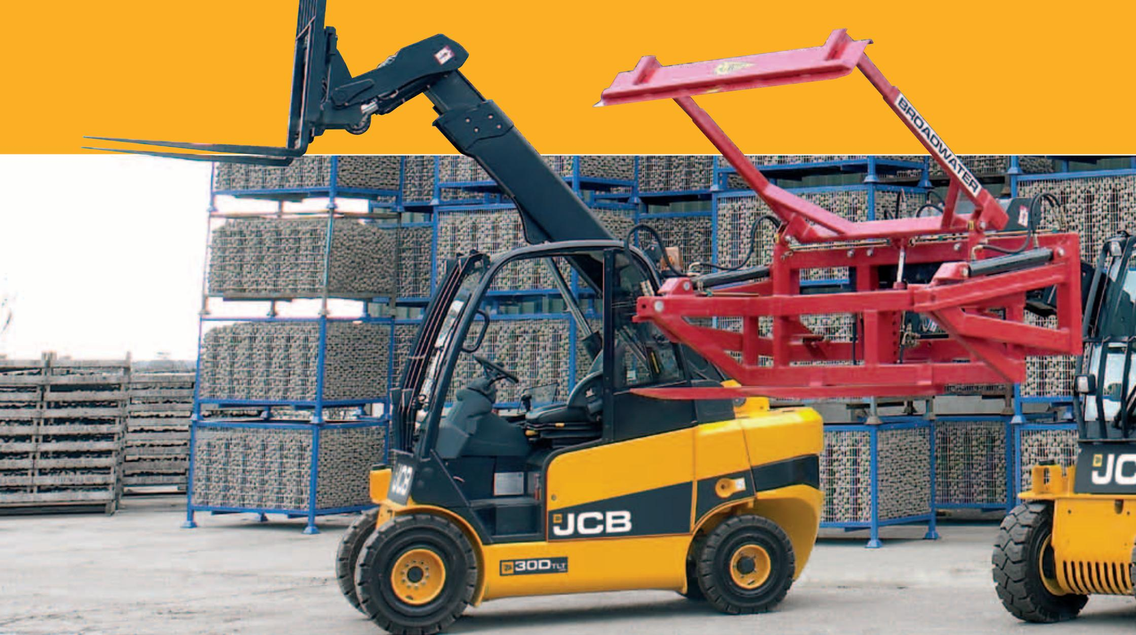
First take the small footprint of an industrial counterbalanced lift truck. Then add the telescopic boom of a telescopic handler. Design-in a fully enclosed hydrostatic drive system. Then finish off with a hydraulic quick-disconnect carriage for forks or shovel. Well that's what we've done at JCB to bring you the JCB Teletruk Range; the world's
