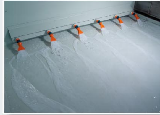
Chip Flushing System Chip flushing system is equipped to remove cutting chips inside of enclosure, which prevents chip accumulation and any possible damage to the linear guideways and ball screws.
